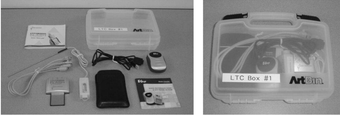
**Figure 15.1** Typical Package Participants Received During Week-Long Handheld Experience. Items include from left to right: Data Harvest Temperature Probe and Data Logger, ArtBin Quick View Storage Box, Toshiba Pocket PC e750 and USB Power Sync Cable, Sandisk 256MB SD Card, and Veo CF Camera.
